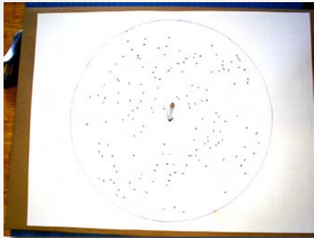
Once the white paper has been inked, the Tines-Template is then once again... painstakingly rotated over the dots. This time, the Sharpie is used to fill in the exact rectangular dimensions for the punch on each occurrence.
